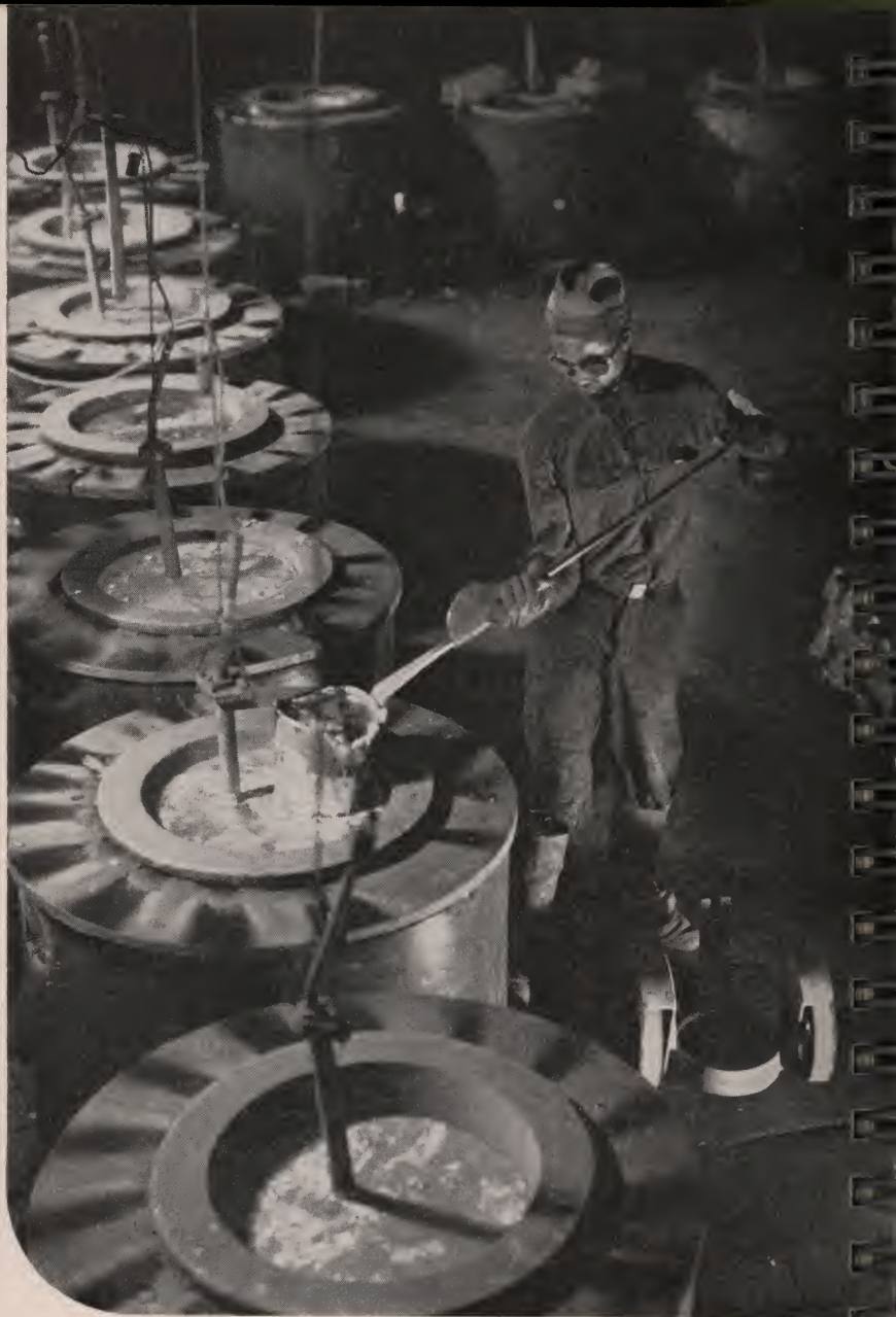
Taking molten aluminum from a holding furnace.
